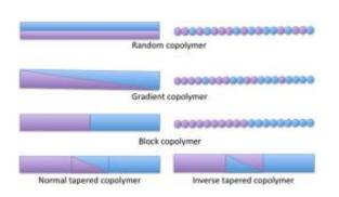
Cartoon of density profile and segment distribution along model polymer chains as a function of position, where purple represents isoprene and blue represents styrene, illustrating the difference between random, gradient, block, and tapered block copolymers.
