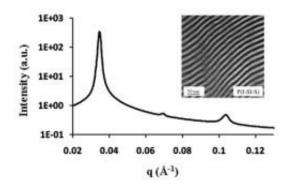
Synchrotron-SAXS data for a P(I-SI-S) tapered diblock copolymer. Specimens were annealed at 210 oC and then cooled to room temperature for data acquisition. The integral moduli values are characteristic of two-domain lamellae. The inset shows a transmission electron microscopy image of a P(I-SI-S) specimen. The sample is stained by OsO4 vapor to enhance contrast.
