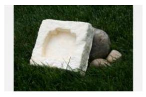
EcoCradle packaging material is composed of agricultural byproducts (cotton gin trash) bound together by fungal mycelium. With an appearance and functionality of polymer foams, EcoCradle can be manufactured with just one eighth the energy and one tenth the carbon dioxide of traditional foam packing material. Credit: Edward Browka, Ecovative Design
