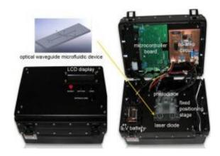
The first prototype of lab-on-a-chip system for detecting microbes in water, food and air. (Photo credit: UA Biosensors Lab)
