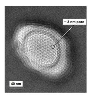
This image, taken by a transmission electron microscope at the University of New Mexico, shows the unique kinked nanopore array platform.
