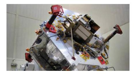
Once the radiation vault was installed on top of the propulsion module, NASA's Juno spacecraft was lifted onto a large rotation fixture to continue with its assembly process. Image Credit: NASA/JPL-Caltech/LMSS
