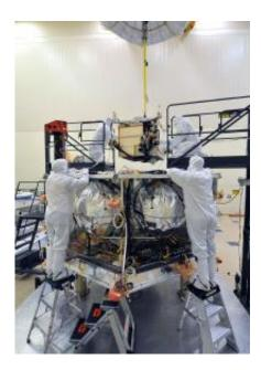
Workers place the special radiation vault for NASA's Juno spacecraft onto the propulsion module. Image Credit: NASA/JPL-Caltech/LMSS
