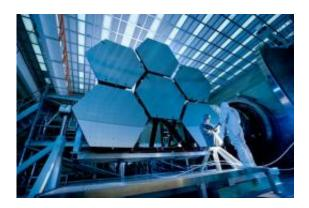
During cryogenic testing, the mirrors will be subjected to temperatures dipping to -415 degrees Fahrenheit, permitting engineers to measure in extreme detail how the shape of each mirror changes as it cools. (NASA/MSFC/David Higginbotham/Emmett Given)
