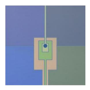
This is a diagram of a NIST ion trap that incorporates an optical fiber to collect light emitted by the ions (electrically charged atoms). Individual electrodes used to trap an ion 30 to 50 micrometers above the surface are shown in different colors surrounding a 50-micrometer-wide hole where light is collected and deposited in a fiber attached below. Credit: A. VanDevender/NIST
