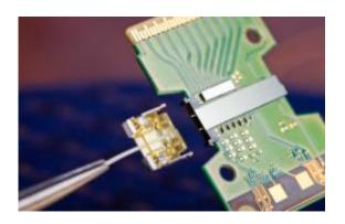
A 50Gbps Silicon Photonics transmit module (left) sends laser light from the silicon chip at the center of the green board, which then travels through optical fiber to the receiver module (right), where a second silicon chip detects the data on the laser and coverts it back into an electrical signal.
