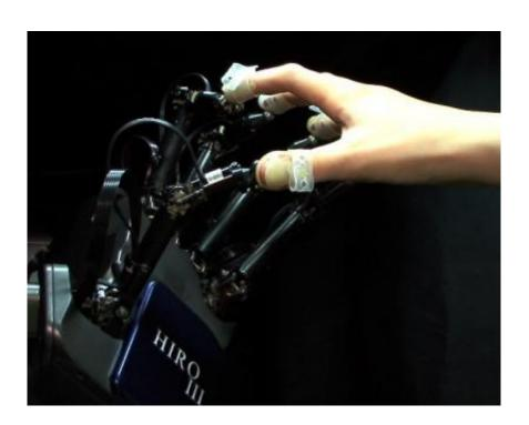
(PhysOrg.com) -- Researchers in Japan are developing a new touch screen system, the HIRO III, that incorporates a robot hand that could offer a new way of simulating the touching of virtual objects and receiving feedback from them.
