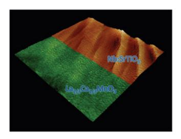
Electronic properties have been measured as function of the distance to the interface between La2/3Ca1/3MnO3 and Nb-doped SrTiO3.
