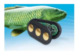
The microsensor system measures the skin resistance, body temperature, blood pressure, heart and respiratory rate of fish. (© Fraunhofer IZM)
