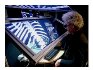
Calit2 Virtual Reality Design Engineer Greg Dawe demonstrates the HUVR device, which combines a consumer 3D HDTV panel, a half-silvered mirror and a touch-feedback controller that allows users to literally 'touch' a generated image as if it was a tangible three-dimensional object.
