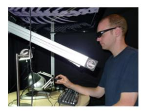
Calit2 VIsualization Specialist Andrew Prudhomme manipulates HUVR's forcefeedback controller. A less expensive, re-engineered version of 30-year-old technology, HUVR could be used to visualize and manipulate a 3-D image of a person's brain taken from an MRI, or an artifact too fragile or precious to be physically handled.
