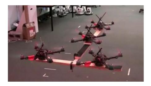
Control of multiple quadrotor robots to cooperatively transport a payload. A gripping mechanism attached to each quadrotor permits grasping of the payload. Work done at GRASP Lab, University of Pennsylvania.
