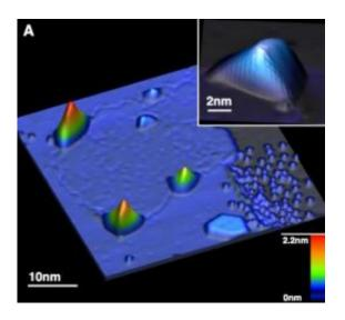
This is a scanning tunneling microscope image of a single layer of graphene on platinum with four nanobubbles at the graphene-platinum border and one in the patch interior. The inset shows a high-resolution image of a graphene nanobubble and its distorted honeycomb lattice due to strain in the bubble. Credit: Crommie lab, UC Berkeley
