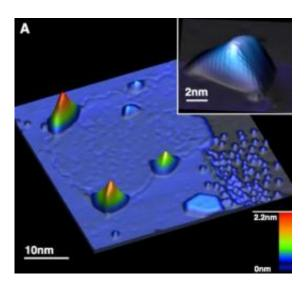
This is a scanning tunneling microscope image of a single layer of graphene on platinum with four nanobubbles at the graphene-platinum border and one in the patch interior. The inset shows a high-resolution image of a graphene nanobubble and its distorted honeycomb lattice due to strain in the bubble. Credit: Crommie lab, UC Berkeley
