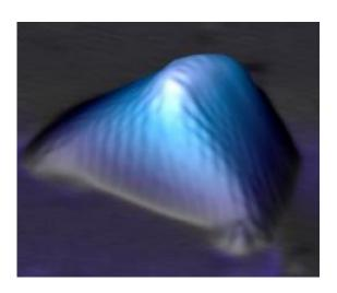
In this scanning tunneling microscopy image of a graphene nanobubble, the hexagonal two-dimensional graphene crystal is seen distorted and stretched along three main axes. The strain creates pseudo-magnetic fields far stronger than any magnetic field ever produced in the laboratory Credit: courtesy of Micheal Crommie, Berkeley Lab
