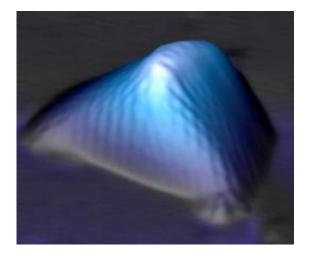
In this scanning tunneling microscopy image of a graphene nanobubble, the hexagonal two-dimensional graphene crystal is seen distorted and stretched along three main axes. The strain creates pseudo-magnetic fields far stronger than any magnetic field ever produced in the laboratory Credit: courtesy of Micheal Crommie, Berkeley Lab
