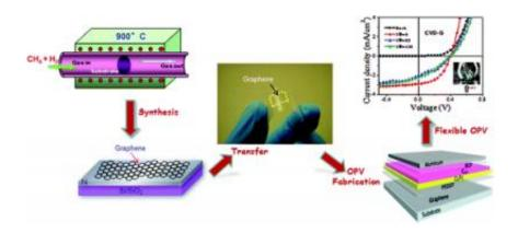
A flow of methane and hydrogen gas mixture deposits carbon atoms as graphene on a nickel plate. The graphene later is then transferred to a plastic sheet, which is then incorporated into an organic photo voltaic (OPV) cell. Credit: USC Viterbi School of Engineering
