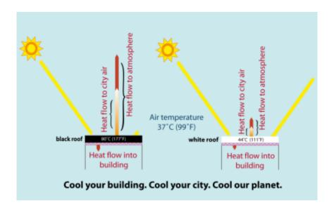
The surface of a black roof (left) heats up 78F above the air temperature, while the surface of a white roof (right) heats up only 12F. Additionally, with a black roof, far more heat flows both to the city and into the atmosphere (arrow lengths are proportional to energy radiated).
