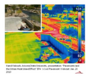
Lighter colored pavement is more reflective, resulting in a cooler surface temperature. (Photo courtesy ASU National Center of Excellence for SMART Innovations)
