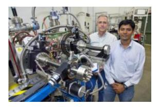
Fundamental research conducted at facilities like Berkeley Lab's Advanced Light Source could lead to the energy-saving technologies of tomorrow, such as a magnetic fridge. Jeff Kortright (left) and Sujoy Roy with an an endstation for soft x-ray resonant magnetic scattering and spectroscopy, which the scientists used at the Advanced Light Source's beamline 4.0.2 to learn more about the magnetocaloric effect in alloys. (Image by Roy Kaltschmidt)
