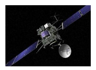
Artist view of ESA's Rosetta cometary probe. The spacecraft is covered with dark thermal insulation in order to keep its warmth while venturing into the coldness of the outer Solar System, beyond Mars orbit. Selected in November 1993 as a cornerstone mission of ESA's long-term science programme, the Rosetta probe was launched by an Ariane 5 on 2 March 2004, on an 11-year journey to the comet 67P/Churyumov-Gerasimenko.
