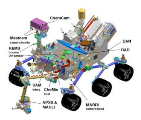
The figure above shows the location of the 10 science instruments on the rover. Image credit: NASA/JPL-Caltech
