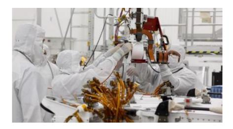
In this image, engineers are dressed head to toe in "bunny suits" (white hoods, lab-style coats and gloves). Only their eyes and foreheads can be seen. They are huddled around the base of the rover's "neck" (its Mast). They watch intently as they carefully lower the Mast to attach it to the rover's flat "back." A cluster of yellow and red wires on the rover's body pokes up in the foreground of the image. Image credit: NASA/JPL-Caltech
