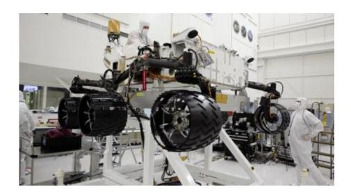
Engineers just installed six new wheels on the Curiosity rover, and rotated all six wheels at once on July 9, 2010. Credit: NASA/JPL-Caltech
