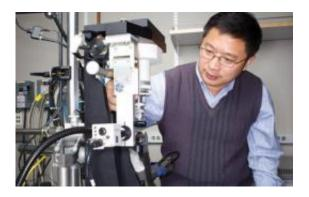
Lin Chen, professor of biological sciences and chemistry, aligns a protein crystal on an X-ray diffractometer. He uses X-ray crystallography to analyze the molecular details of key proteins and their complexes in physiological and disease processes. Photo credit Max S. Gerber.
