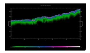
One of CryoSat-2's first synthetic aperture radar data images shows a track across central Antarctica -- an area never before charted by satellite. The fine structure in the ice surface, which would be blurred in data acquired by a conventional radar altimeter, is clearly visible. Credit: ESA
