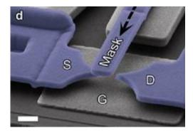
The innovative transistor with contacts (S, D), the substrate acting as gate (G) and the shadow mask shielding the carbon nanotube during vapour-deposition of the contact metal. (Photo: M. Muoth / ETH Zurich)
