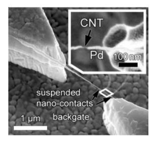
A single carbon nanotube (CNT) is grown between two contacts. The ends were coated by vapour-deposition of palladium to connect to the suspended transistor channel. (Photo: M. Muoth / ETH Zurich)
