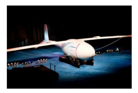
The Boeing Company today unveiled the hydrogen-powered Phantom Eye unmanned airborne system, a demonstrator that will stay aloft at 65,000 feet for up to four days.
