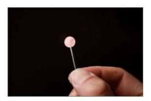
This dime-sized coin made of aluminum and copper is used to induce short circuits in lithium-ion batteries. The ability to induce shorts on demand is crucial to finding out how hot a battery can get when it fails while in active use. Credit: Pat Corkery
