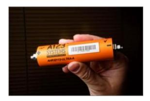
This prototype lithium-ion battery for automobiles has the advantage of being lighter and taking up far less room than the batteries now in hybrid cars. Credit: Pat Corkery
