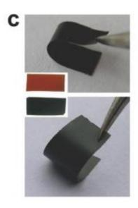
A new form of paper made of super-thin sheets of carbon could help fight disease-causing bacteria in applications ranging from anti-bacterial bandages to food packaging. Credit: ACS Nano
