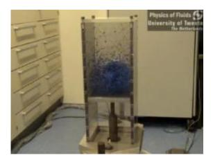
This image from the video below shows the machine that uses bouncing beads to perform work, confirming a thought experiment from 1912. Credit: University of Twente.
