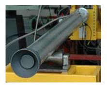
An off angle view of the ED nozzle attached to the combustion chamber of a test hybrid rocket motor, with the central plug / pintle prominent. The rocket motor is being tested by Airborne Engineering and the University of Bristol in the J1 static test firing cell.
