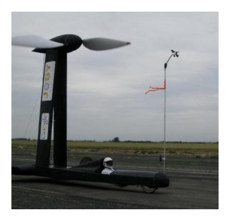
Cavallaro explained the car is able to move faster than the wind because the propeller is not turned by the wind. The wind pushes the vehicle forward, and once moving the wheels turn the propeller. The propeller spins in the opposite direction to that expected, pushing the <u>wind</u> backwards, which in turn pushes the <u>car</u> forwards, turning the wheels, and thus turning the propeller faster still.
