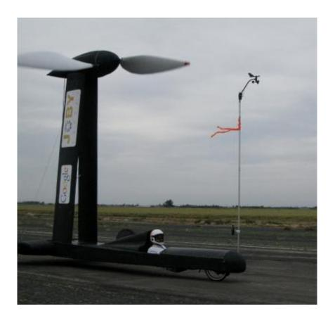
Cavallaro explained the car is able to move faster than the wind because the propeller is not turned by the wind. The wind pushes the vehicle forward, and once moving the wheels turn the propeller. The propeller spins in the opposite direction to that expected, pushing the wind backwards, which in turn pushes the car forwards, turning the wheels, and thus turning the propeller faster still.
