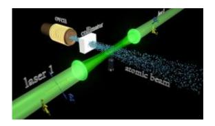
Two opposed laser beams, identical except for polarization, attempt to excite forbidden two-photon transitions in a beam of barium atoms. (Image Damon English)
