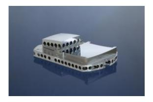
The M2/M3 assembly with two exactly aligned aspherical mirrors from the IRS-Tel reflecting telescope was produced with extremely high precision by using additional reference marks. (© Fraunhofer IOF)
