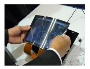
At the SID 2010 Toshiba demonstrated their LCD panel that can be bent to zoom in-and-out of displayed images. Credit: Toshiba Corp.
