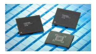
Toshiba Launches Industry's Largest Embedded NAND Flash Memory Modules. e •MMCTM Compliant Embedded Memories Combine up to 128GB NAND and a Controller in a Single Package. Credit: Toshiba Corp.
