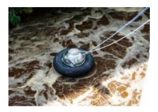
Online real-time measurement of N2O and nitrogen oxide from biological wastewater treatment plants is conducted using a new U.S. EPA-reviewed protocol developed by Columbia researchers that employs a floating surface emission flux chamber, as shown in this image. Image credit: Kartik Chandran
