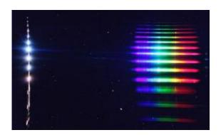
The students recorded this spectrum of the disintegrating spacecraft. The colors reveal much about the response of Earth's atmosphere to the hypervelocity spacecraft and how the spacecraft itself was breaking up.
