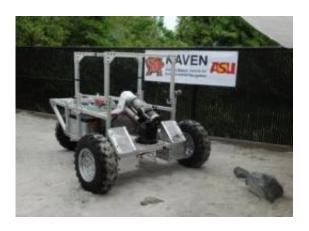
The lunar concept of RAVEN, the 3-wheeled rover with an arm, would have a mass of ~150 kg (~330 lbs for Earth) and the Earth-analog prototype is ~340 kg (~750 lbs for Earth). Credit: Courtesy of Project RAVEN team ASU/UMd.
