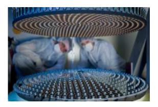
A picture of the movable secondary mirror during its installation in the Arcetri lab. The image shows the 672 tiny magnets spread over the back of the mirror. The reflecting face of the mirror is face down. The upper portion contains the electro-mechanical devices that control the magnets. Image: LBT Collaboration / R. Cerisola
