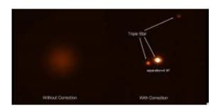
A double star as observed with the LBT in standard mode (left), and with the adaptive correction activated (right). Because of atmospheric blurring, the fainter companion of the star cannot be identified in the images taken in standard mode, while it is easily visible when the adaptive module is activated. A third faint star also becomes visible in the upper right part of the frame, thanks to the increased sensitivity of the telescope in adaptive mode. Image: LBT Collaboration
