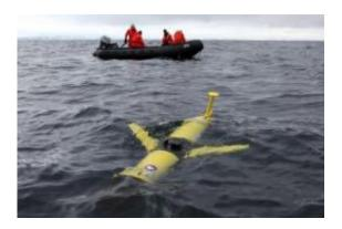
A Rutgers/Webb SLOCUM glider is deployed from a Zodiac near Palmer Station Antarctica. Automated glider robots can measure ocean characteristics continuously for weeks at a time. Credit: Jason Orfanon
