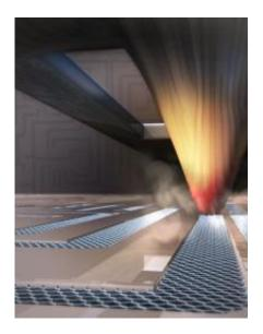
In a technique known as thermochemical nanolithography, the tip of an atomic force microscope uses heat to turn graphene oxide into reduced graphene oxide, a substance that can be used to produce nanocircuits and nanowires with controllable conductivity. Image Credit: University of Illinois at Urbana-Champaign
