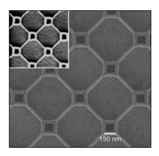
A fragment of a superconducting thin film patterned with nano-loops measuring 150 nanometers on a side (small) and 500 nanometers on a side (large), where the nano wires making up each loop have a diameter of 25 nanometers.
