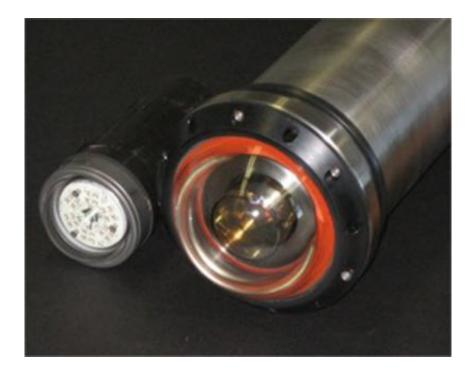
The prototype optical modem is comprised of a small LED transmitter (left) with a photo-multiplier receiver, providing low-power, multipoint bi-directional communications over distances of up to 200 meters. (Woods Hole Oceanographic Institution)
