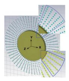
The design of the invisibility cloak consists of a spoke-like configuration of glass resonators, which form a magnetic resonance that is used to obtain the desired parameters of the medium. The illustration shows the glass cloak designed to hide a metal cylinder of 15 micrometers in diameter. Image credit: Semouchkina, et al.
