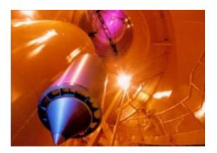
Experiment with a dramatic fall: The capsule is pulled up to the starting position in the drop tower, where the physicists generate a Bose-Einstein condensate by remote control and observe how it behaves at zero gravity -- a step towards extremely-sensitive measuring devices for gravitation. Credit: Image: ZARMS / University of Bremen
