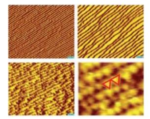
In these STM images of a platinum catalyst, (A) shows the terraced the surface under ultrahigh vacuum, (B) as the surface is covered with carbon monoxide and pressure increases, the terraces widen (C) when coverage is complete and press reaches one torr, the terraces fracture into nanoclusters (D) enlarged view shows triangular shape of the nanoclusters, two of which are marked by red lines. Credit: (Image courtesy of Berkeley Lab Somorjai and Salmeron, et. al)
