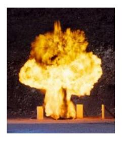
This image shows a detonation within a blast resistant trash receptacle using a large C4 explosive charge. By regulating the explosive force carefully over a series of tests like this one, the research and development team created a scalable blast resistance standard, which can help in comparing a threat assessment with the protection that different trash receptacles provide. Credit: NIST
