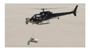
This test of the radar system to be used during the August 2012 descent and landing of the NASA Mars rover Curiosity mounted an engineering test model of the radar system onto the nose of a helicopter. Image Credit: NASA
