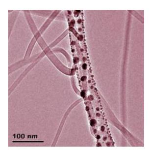
Under the transmission electron microscope (TEM), several cobalt phthalocyanine nanowires grow out of an iron phthalocyanine nanowire which is decorated with silver particles. Credit: Empa
