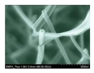
Under the scanning electron microscope (SEM), palladium octaethyl-porphyrin nano-lamellae and nanowires grow on a perylene nanowire which has been sputtered with silver particles. Credit: Empa
