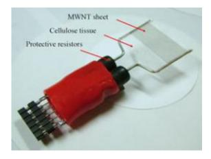
Thin, almost transparent sheets of multi-walled (MWNT) nanotubes are connected to an electrical source, which rapidly heats the nanotubes causing a pressure wave in the surrounding air to produce sound.
