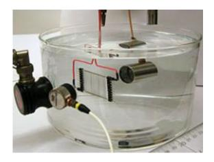
An experimental setup measures acoustic sound projection in liquids from a sheet of carbon nanotubes.
