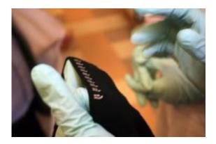
Chemical-sensing electrodes printed directly on the inside elastic waistband of underwear. Photo credit: UC San Diego / Daniel Kane
