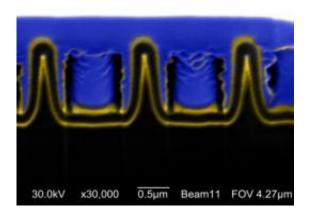
Boston College researchers report developing a "nanocoax" technology that can support a highly efficient thin film solar cell. This image shows a cross section of an array of nanocoax structures, which prove to be thick enough to absorb a sufficient amount of light, yet thin enough to extract current with increased efficiency, the researchers report in the journal *Physica Status Solidi*. Credit: Boston College
