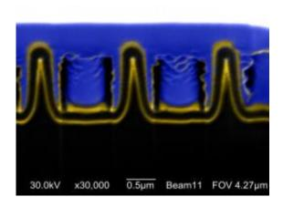
Boston College researchers report developing a "nanocoax" technology that can support a highly efficient thin film solar cell. This image shows a cross section of an array of nanocoax structures, which prove to be thick enough to absorb a sufficient amount of light, yet thin enough to extract current with increased efficiency, the researchers report in the journal *Physica Status Solidi*. Credit: Boston College
